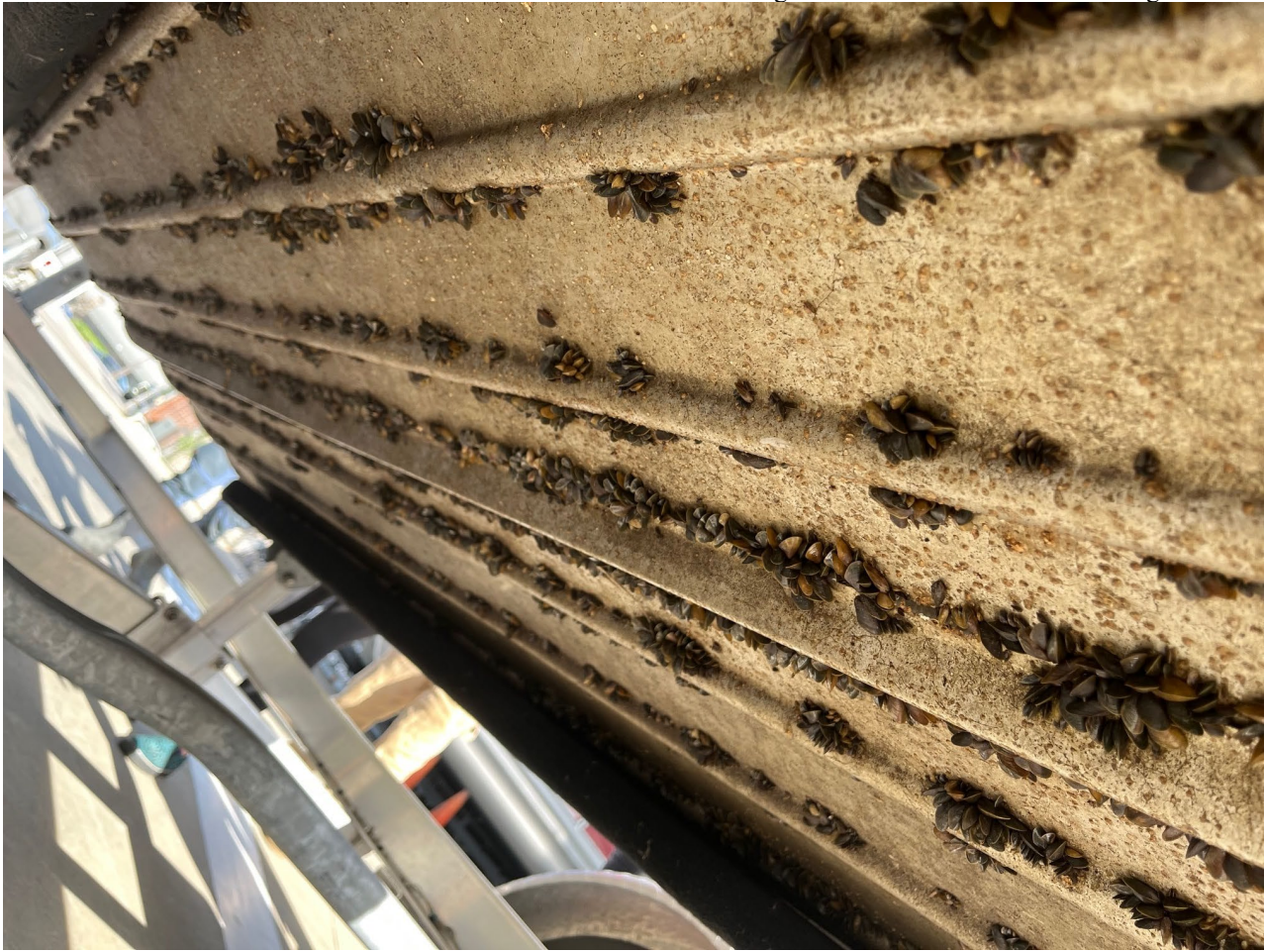
Photo of Hull of Infested Vessel at the Delta - Golden Mussels attached along the underside of a vessel including in linear seams.
