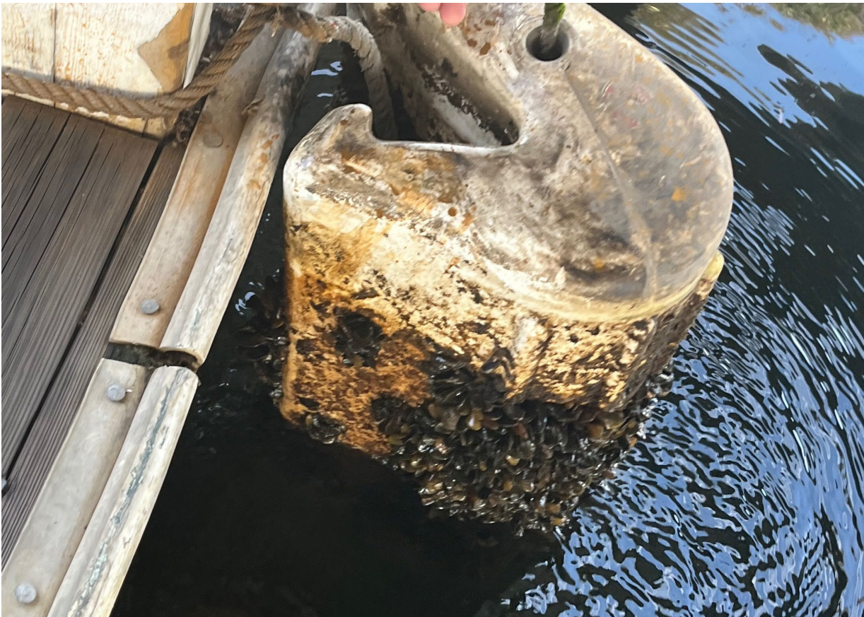
Photo of submerged Buoy with Golden Mussel Infestation – Delta Marina. Example of colonization on dock infrastructure and floating equipment.
