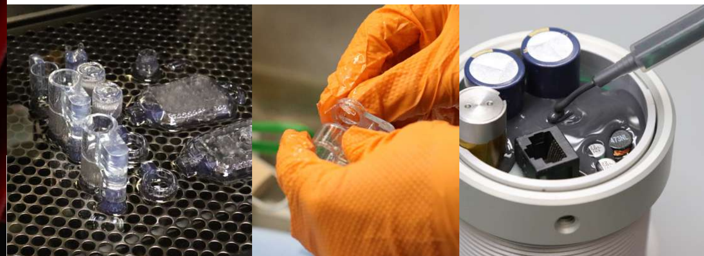
Left to right: 3D printing prototype CyberKey, Developing prototype CyberLock cylinder part, Potting CyberKey Vault (FS-CV01) circuit board.
